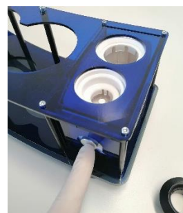
4) Push the humidifier out of the housing
