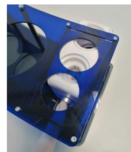
4) Push the humidifier out of the housing
