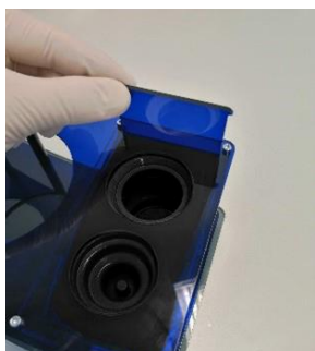
3. Remove the rack lid by pulling up
