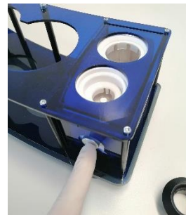
4) Push the humidifier out of the housing
