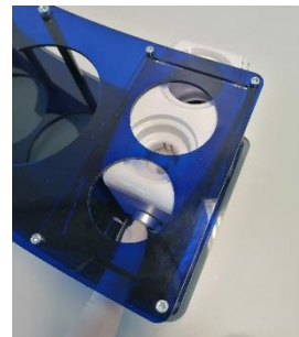
4) Push the humidifier out of the housing
